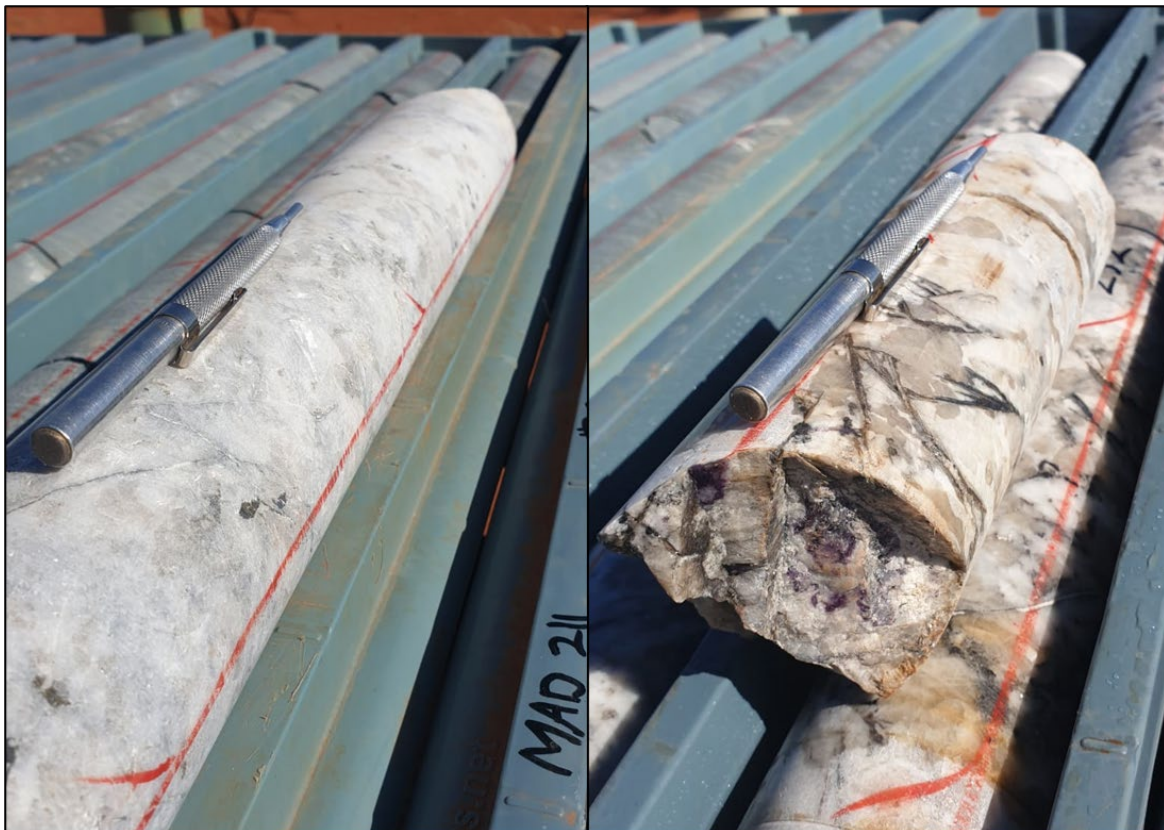
Figure 2 – drill core from MAD 211 showing pegmatite with lithium-bearing minerals. MAD211 intersected six pegmatite intervals that comprised 17.2-18m, 27.6-29.11m, 140.8-143.2m, 230.68-232.4m, 247.75-249.85m and 261.3-262.3m
