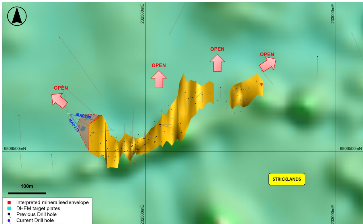
Figure 2 - plan view map (against magnetic data) with schematic of the mineralised envelope at Stricklands. The location of MAD209 and MAD210 is shown and the interpreted extension of the mineralised envelope to the north-west is highlighted.
