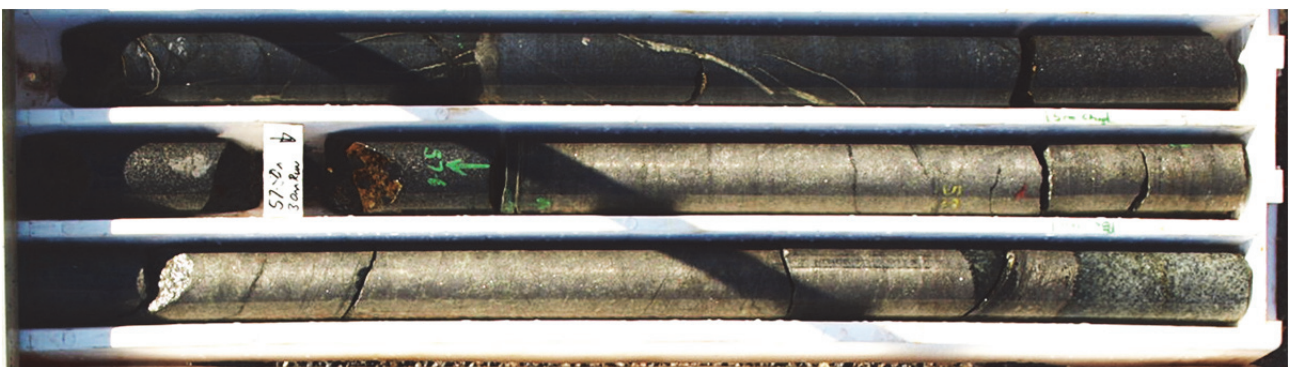
Figure 2 – high grade nickel-copper sulphides in ultramafic on contact with granite in MAD13 drilled by BHP Billiton in 2008 at Cathedrals. The interval highlighted in this photo recorded 1.4m @ 7.1%Ni, 3% Cu and 4.2g/t PGEs from 57.6m. There is strong potential for further intersections of high grade mineralisation in the 2016 planned drilling at Mt Alexander.
