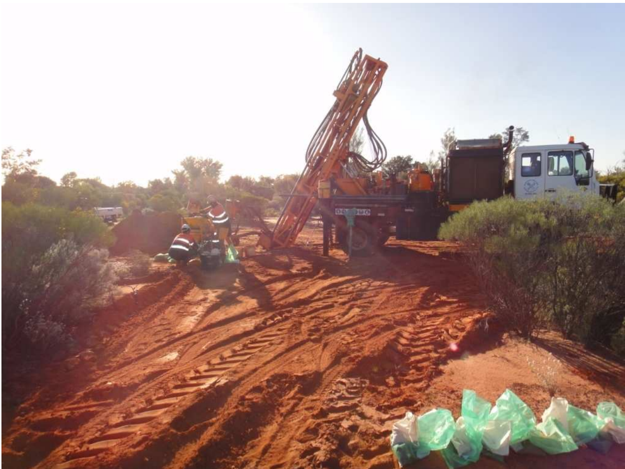
Figure 1 - The air core rig at Hole 18 of the Desert Dragon Prospect
