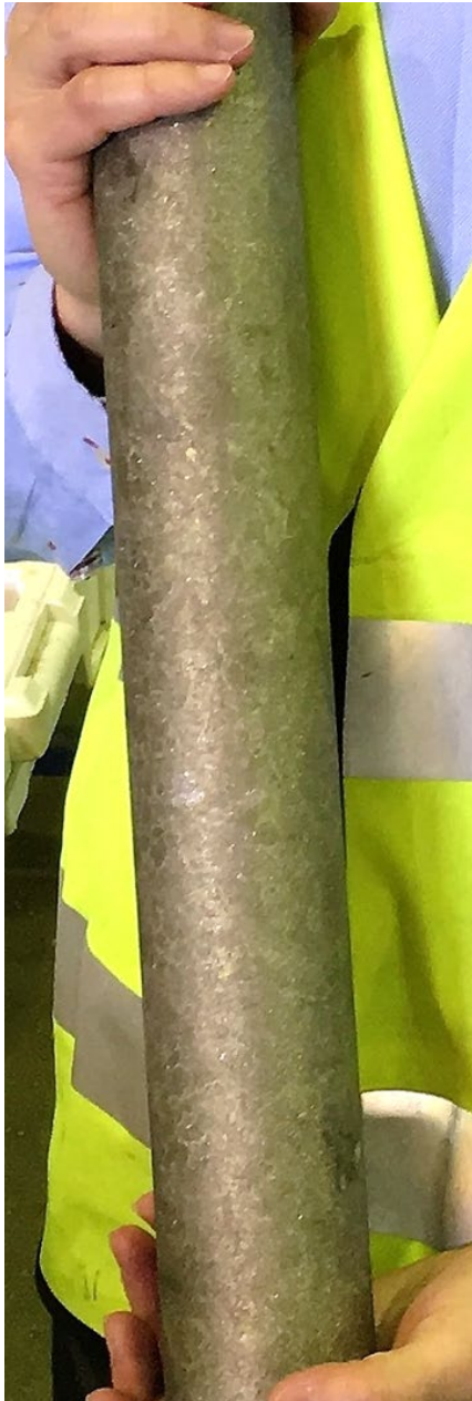
Figure 5 – drill core from MAD56 at the Cathedrals Deposit, showing high-grade massive nickel-copper sulphides
