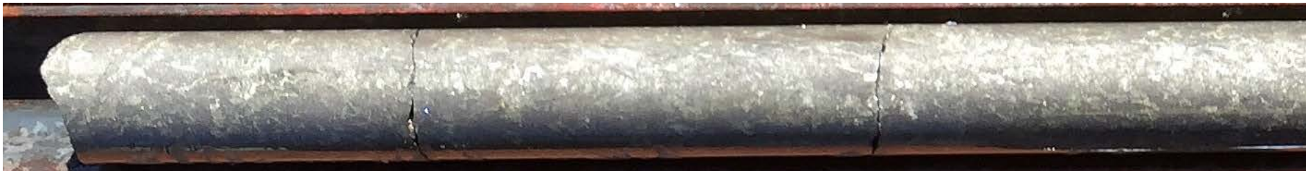
Above: part of the massive nickel-copper sulphide intersection in MAD40 that graded 7.88%Ni and 3.11%Cu
