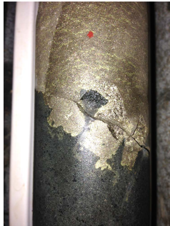
Above: drill core from MAD23 at 57m showing contact of massive nickel-copper sulphides with footwall mafic rocks
