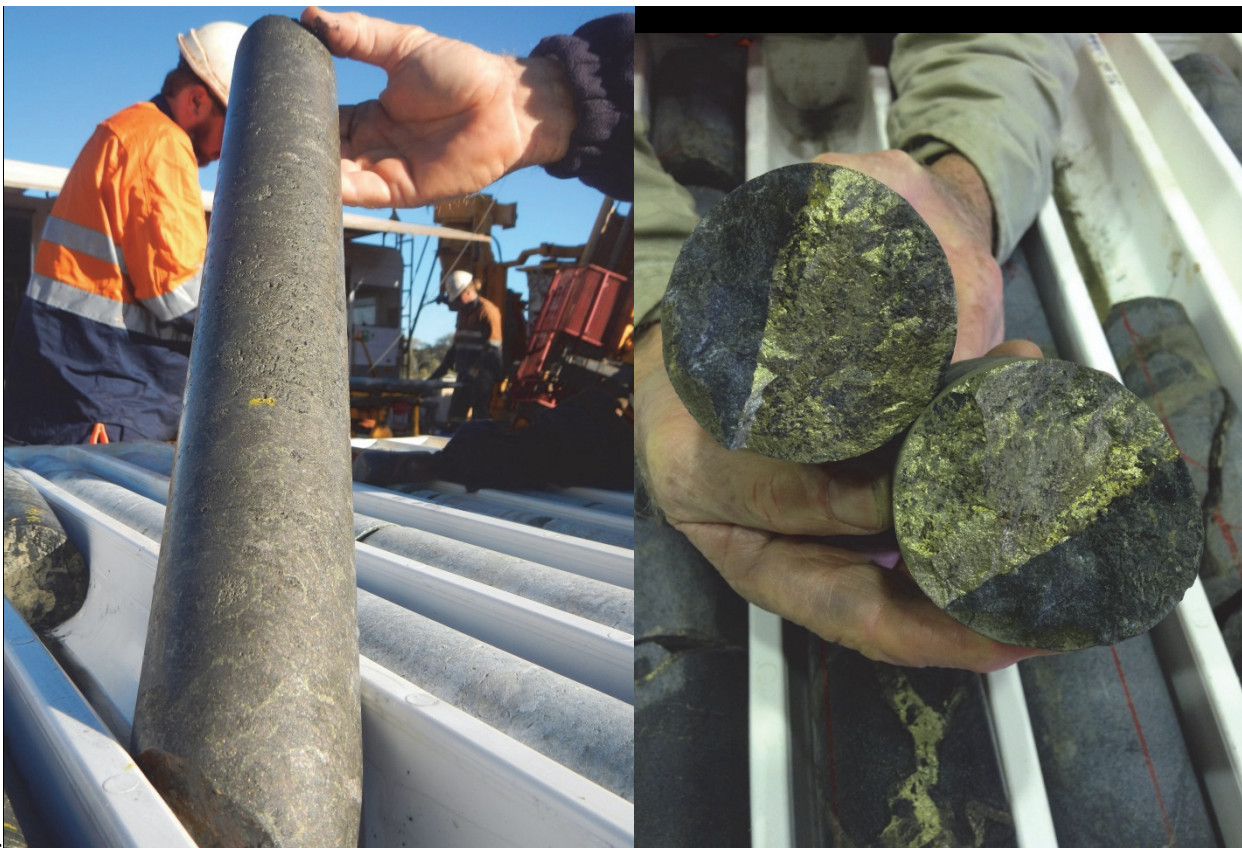
Figure 1 – on left: photograph of drill core from MAD15 interval between 30.17m to 31.34m. Core comprises massive nickel-copper sulphides (pentlandite, chalcopyrite) with 8.75%Ni, 3.37%Cu, 0.24%Co and 6.16g/t total PGEs ; on right: drill core from MAD22 with massive chalcopyrite (yellow-green) in contact with ultramafic (dark grey). Assays for this interval (52.4m to 52.63m) returned 13.1%Cu and 43g/tAg.
