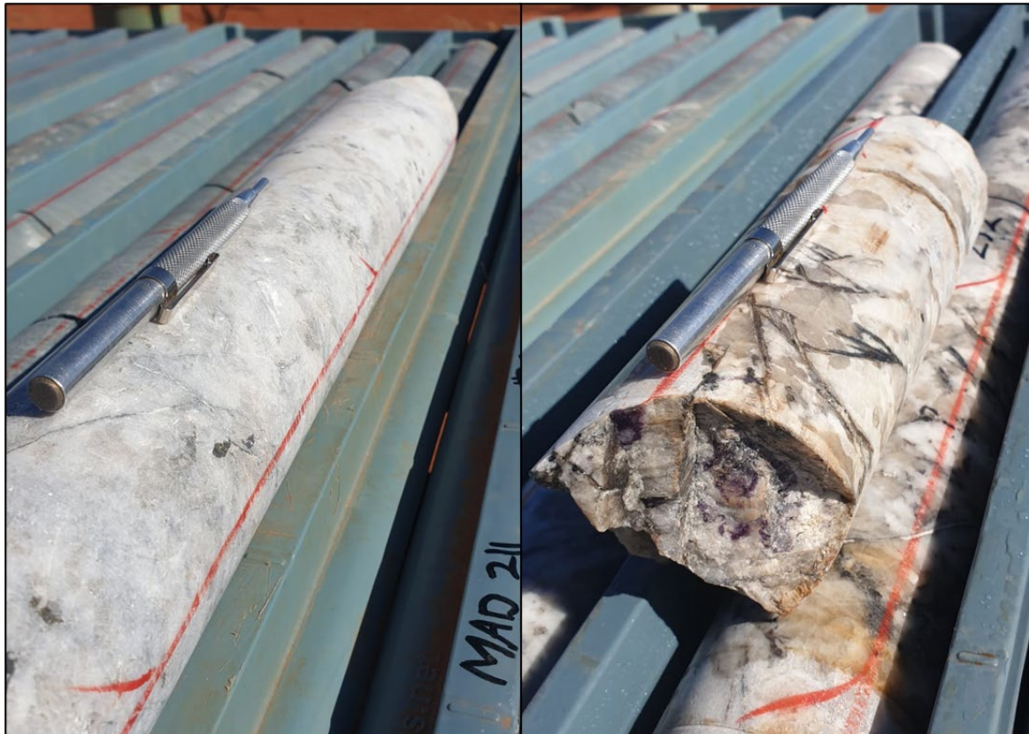
Figure 3 – drill core from MAD 211 showing pegmatite with lithium-bearing minerals.
