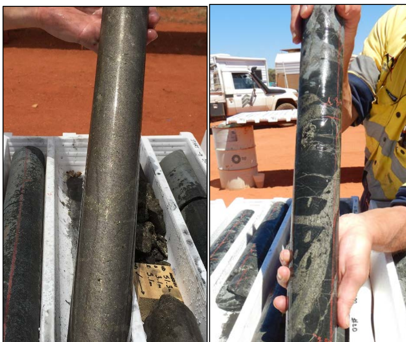
On right: drill core from MAD78 that was drilled 20m to the north of MAD71. Nickel-copper sulphide veinlets and brecciated massive sulphide clasts in the drill core indicate structural influence on the mineralisation remobilised from an in situ massive sulphide source.
