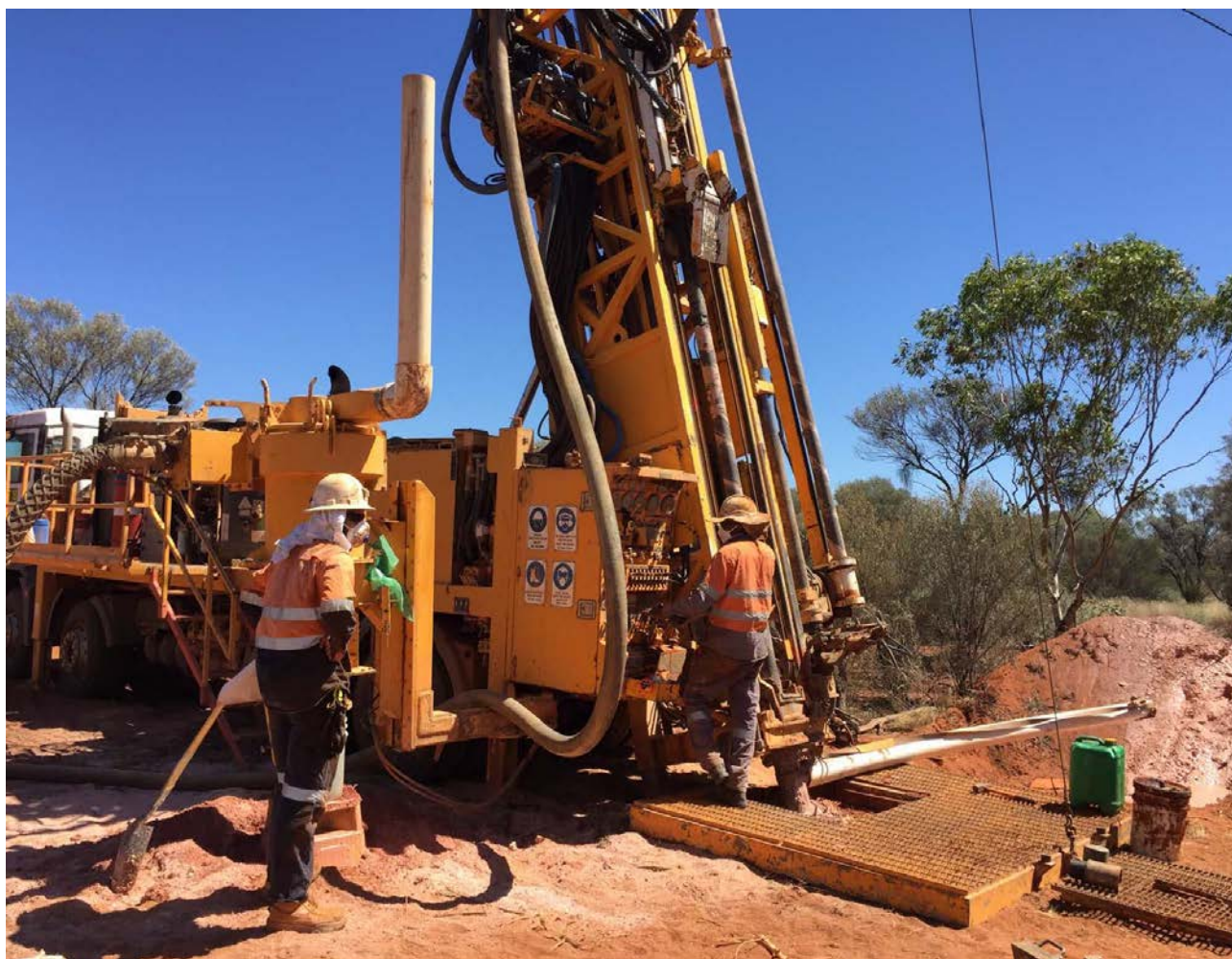
Figure 5 – drill rig at the Mt Alexander Project completing the first RC drill hole listed in Table 1
