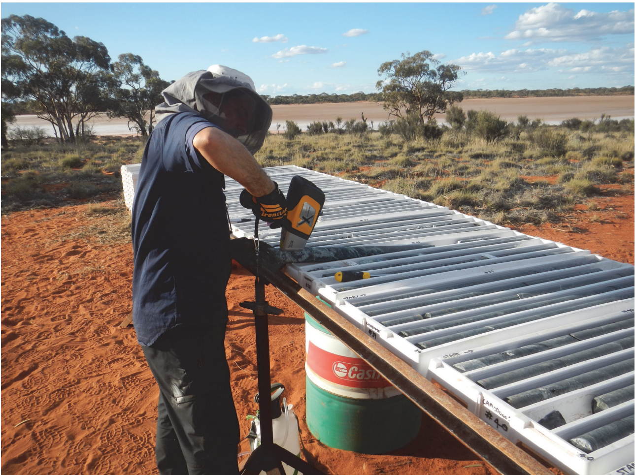
Figure 2 – XRF analysis underway on the drill core from CAMDD001
