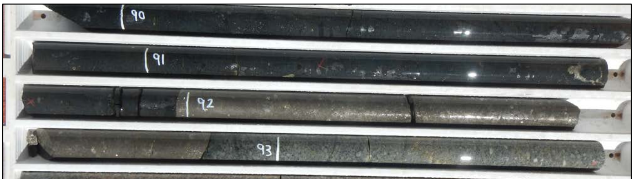
Figure 4 – photograph of drill core from MAD48 showing massive nickel-copper sulphides from 91.98m to 92.89m.
