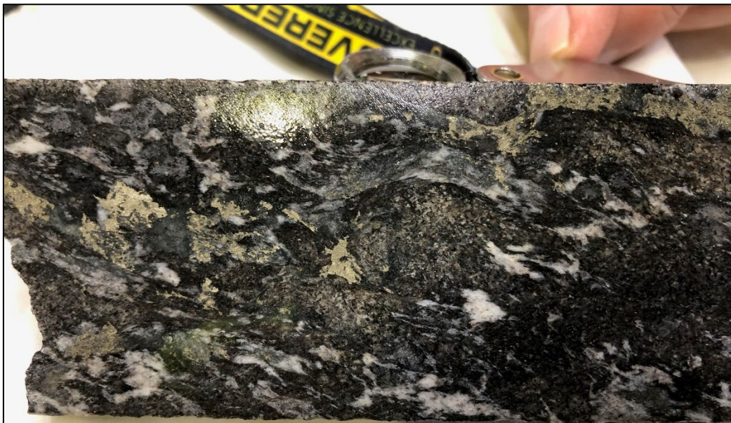
Figure 2 – Core from PDD002 at 236m downhole showing disseminated and semi-massive sulphide as void infill within an interpreted strongly altered breccia.
