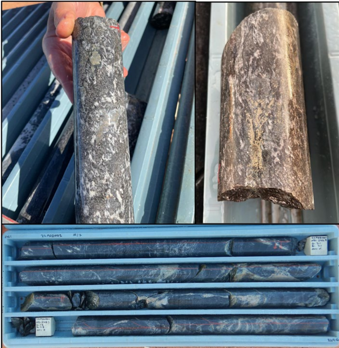
Figure 5 – sulphidic intersections from PDD002 at 235m (top left) and 267m (top right). Structural complexity and alteration of vein sets shown in core tray for PDD001 (bottom).
