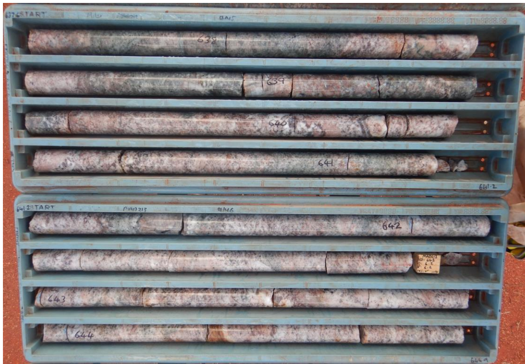
Figure 3 – MAD213 from 637.60m to 644.90m showing a portion of the 120m+ intersect of coarse-grained pegmatite from the Manta seismic reflector
