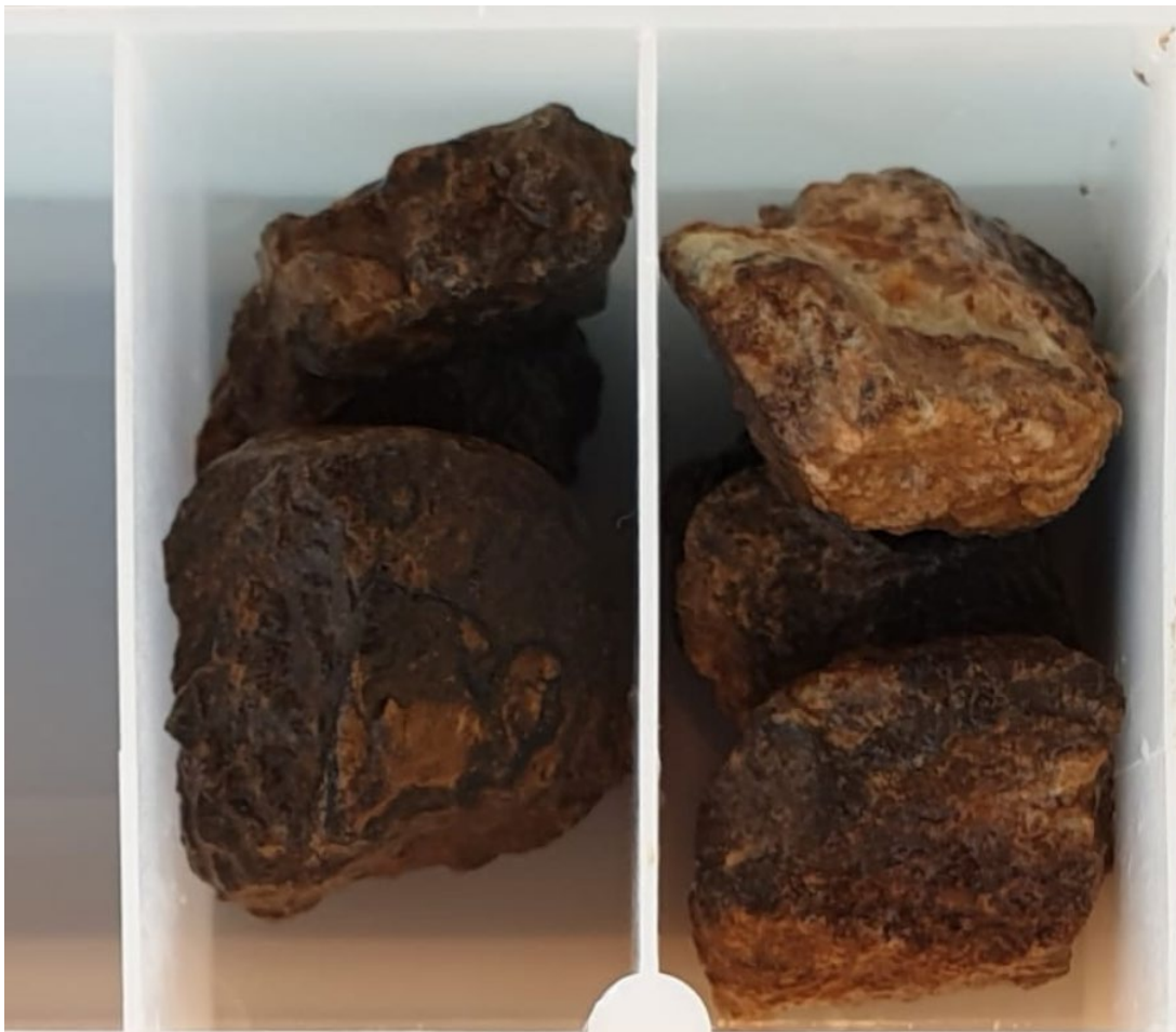
Figure 2 – Photo of drill chips from PRC002 showing ferruginous textures and iron oxides (photo colours not altered).
