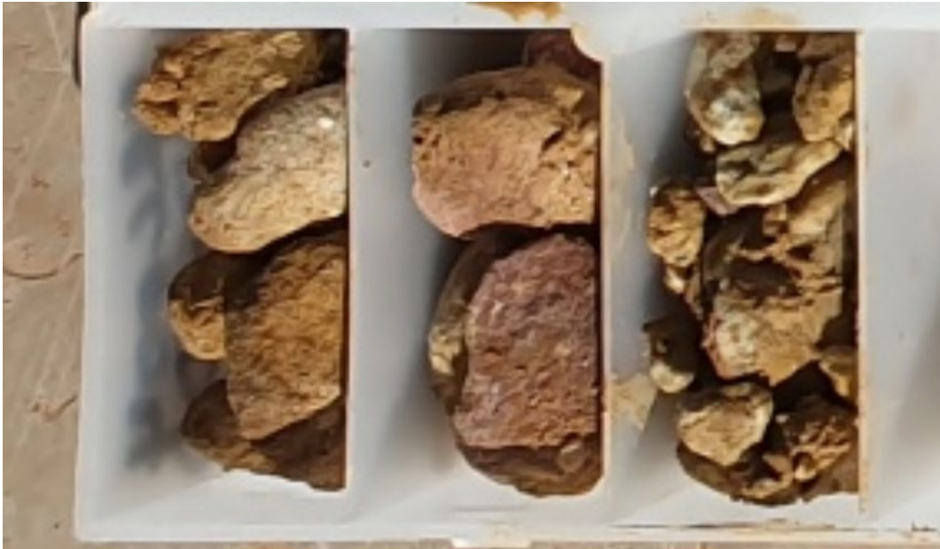
Figure 3 – Photo of drill chips from PRC004 showing weathered and ferruginous basement rocks (photo colours not altered).
