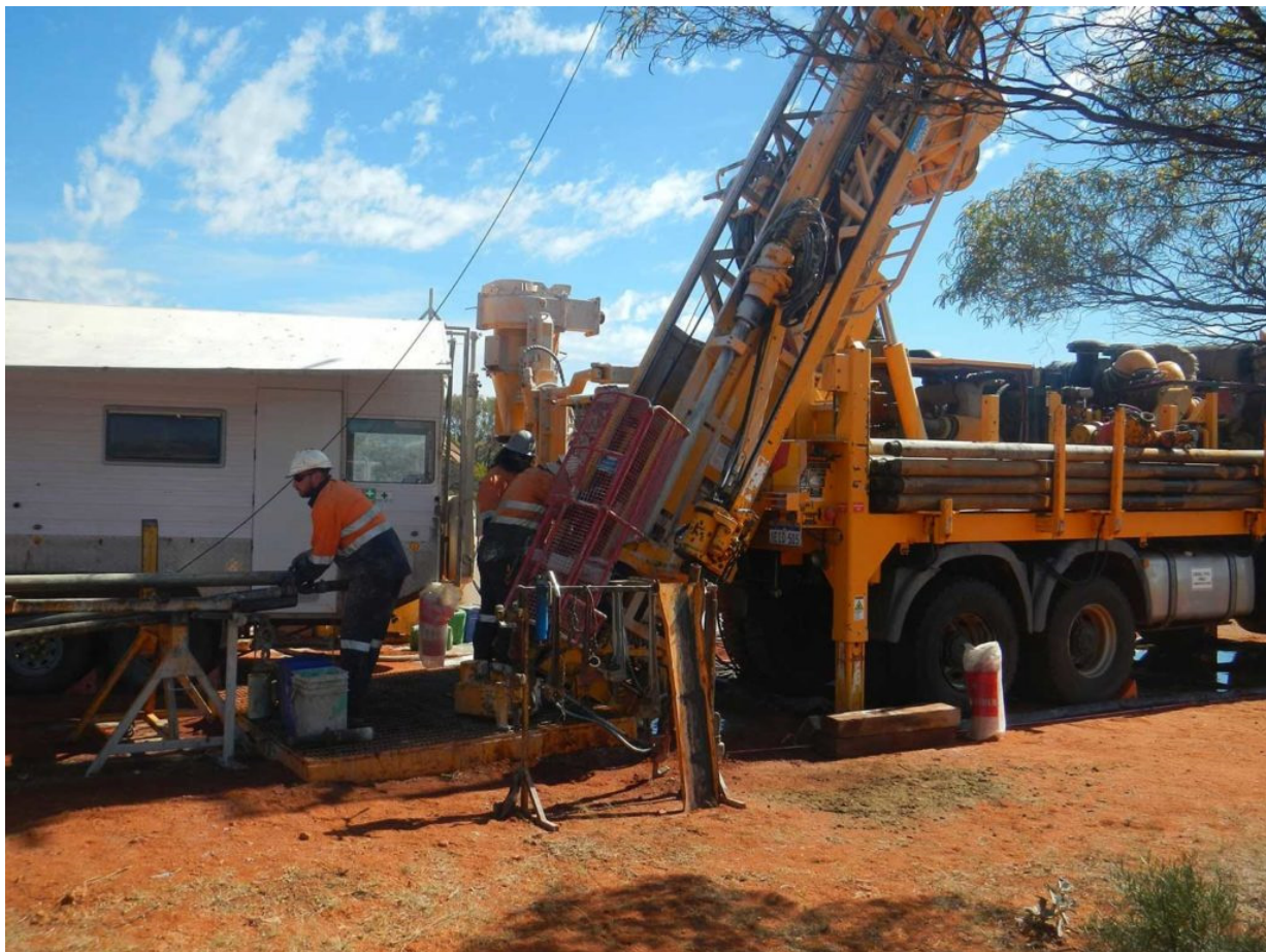
Diamond drilling at Mt Alexander to test for massive nickel-copper sulphides
