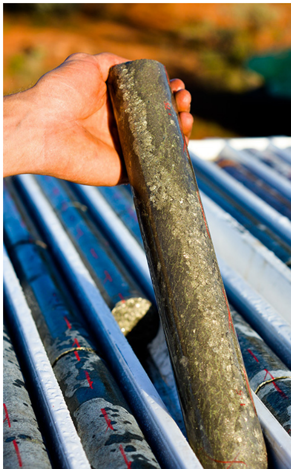
Drill core at Mt Alexander with pure pentlandite analysed at 28% Ni
