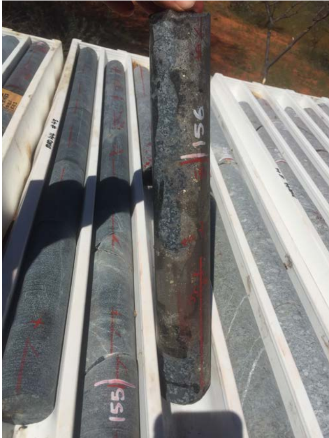
Figure 3 – massive nickel-copper sulphides in MAD44 which included pentlandite-rich rims that recorded 27%Ni in spot XRF readings.
