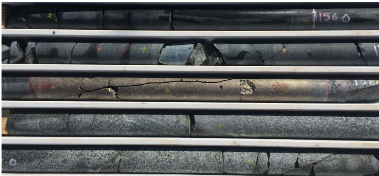
Figure 2 – photograph of drill core from MAD43 showing massive nickel-copper sulphide interval from 157.22m to 157.95m below ultramafic with blebby sulphides.
