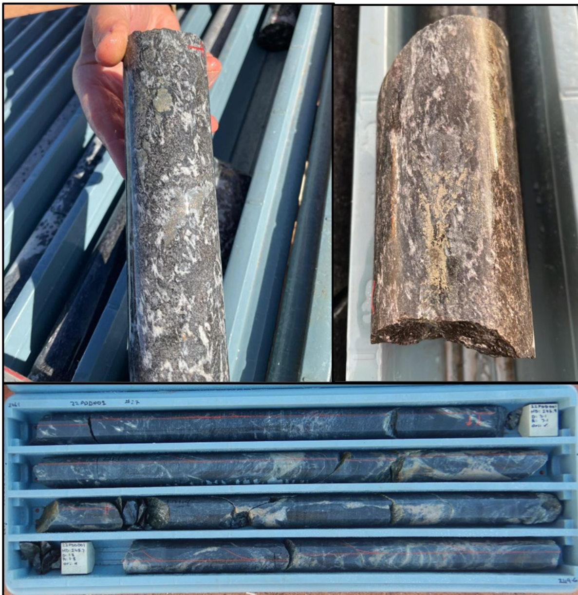
Figure 4 – sulphidic intersections from PDD002 at 235m (top left) and 267m (top right). Structural complexity and alteration of vein sets shown in core tray for PDD001 (bottom).
