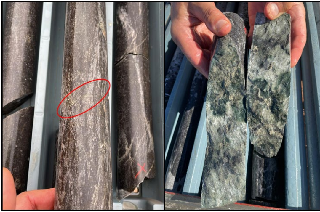
Figure 1 – photos of sulphidic zones within drill core of PDD002, chalco-pyrite (copper sulphide) circled.
