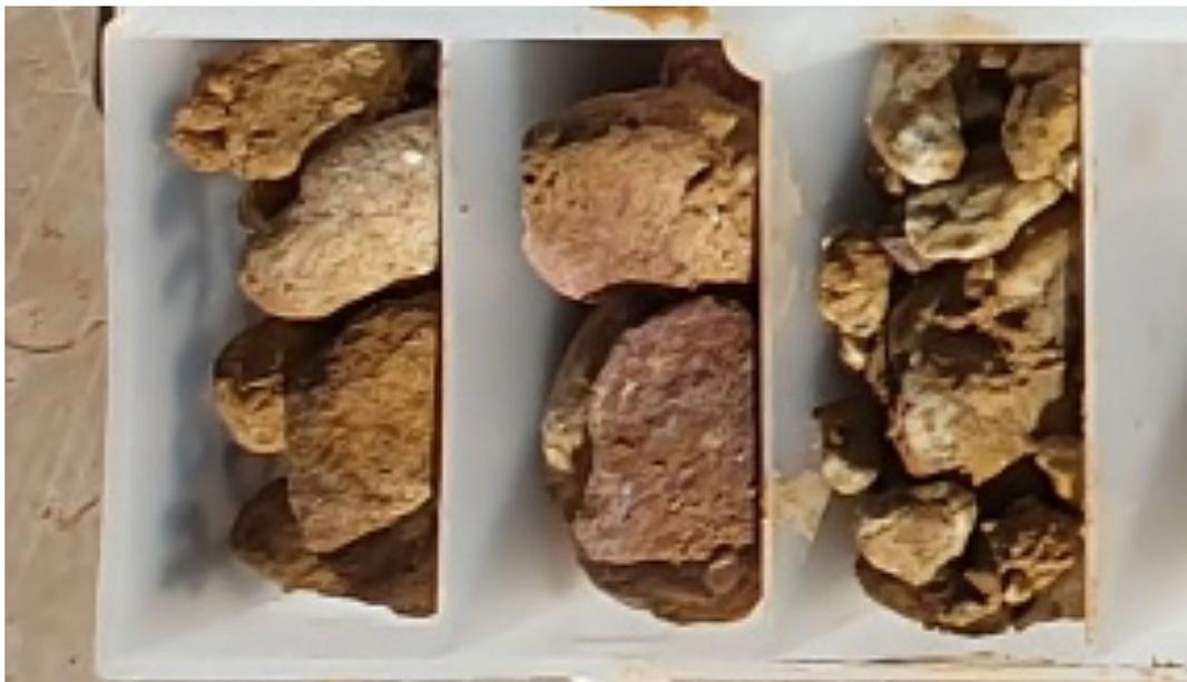
*Figure 5 – Photo of drill chips from PRC004 showing weathered and ferruginous basement rocks (photo colours not altered).*
