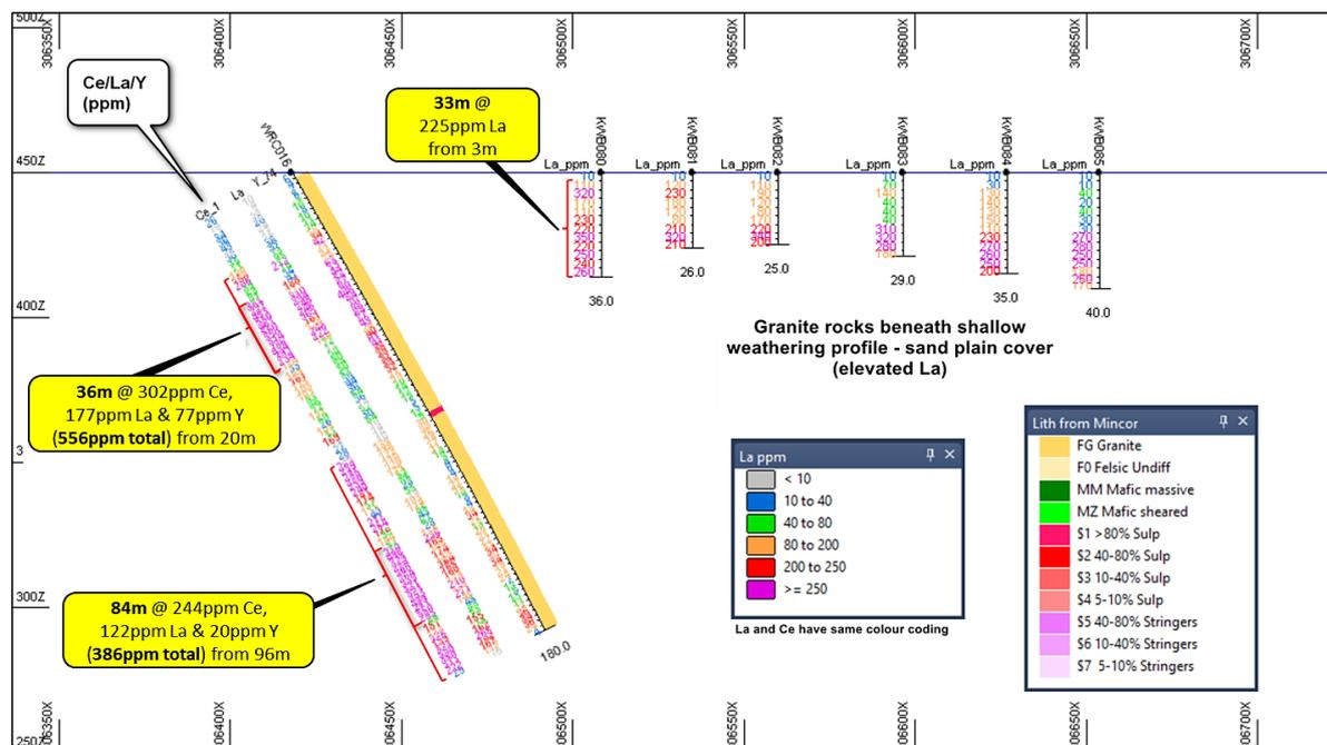
Figure 2: section showing REE anomalism (sourced from Mincor's ASX December Quarterly Report 2010 and GSWA open file report A90100). \*Note, the Cerium maximum cut-off is 500ppm used for calculations based on the assay analysis performed.
