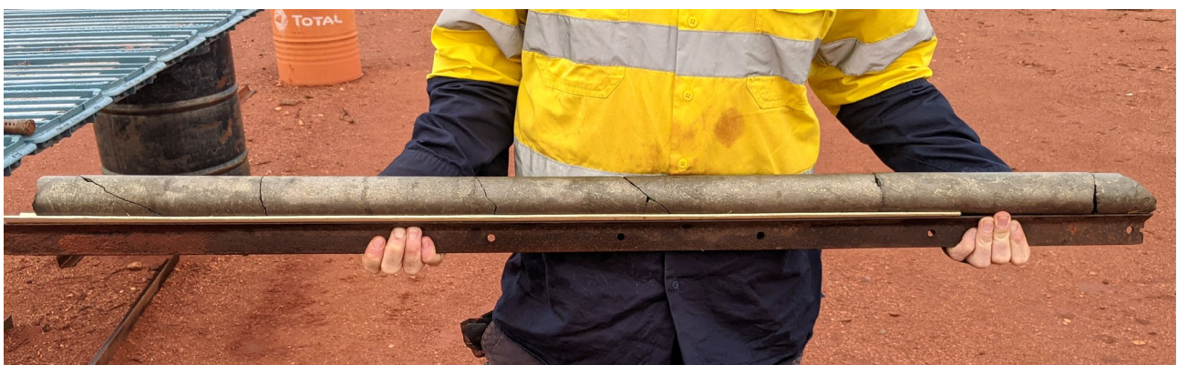
Figure 1 – drill core from MAD199 showing massive nickel-copper sulphides 342.12m to 343.4m downhole
