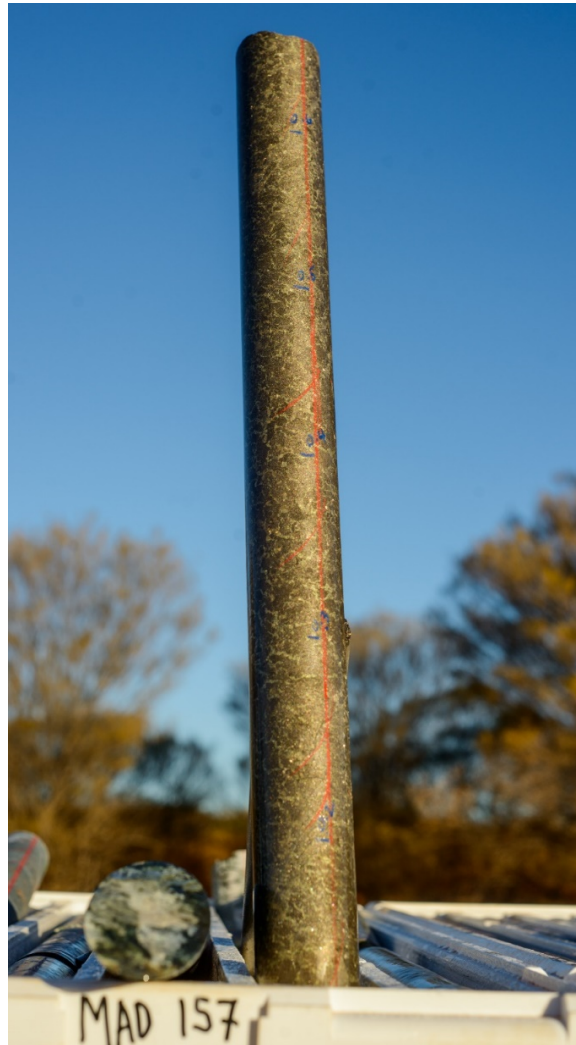
Above: photo of drill core with massive nickel-copper sulphides in MAD157 at 195.84m downhole
