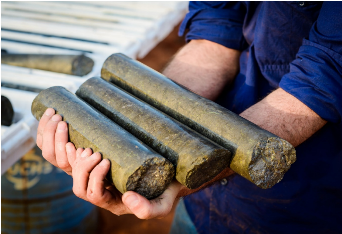
Figure 1 – drill core from MAD152 with massive sulphides that returned assays of 4.29% Ni, 1.46% Cu and 3g/t PGEs from 49.05m
