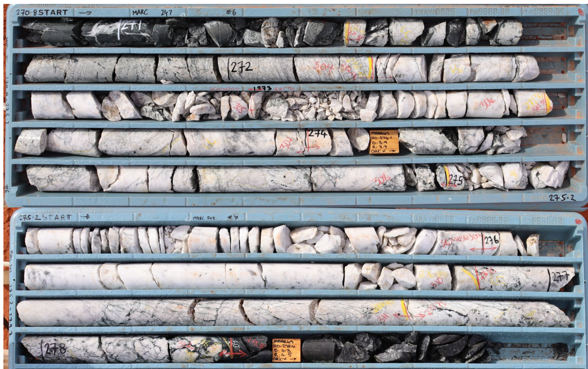
Figure 1 – MARD247 drill core showing pegmatite from 271.25m to 278.35m (awaiting assays).
