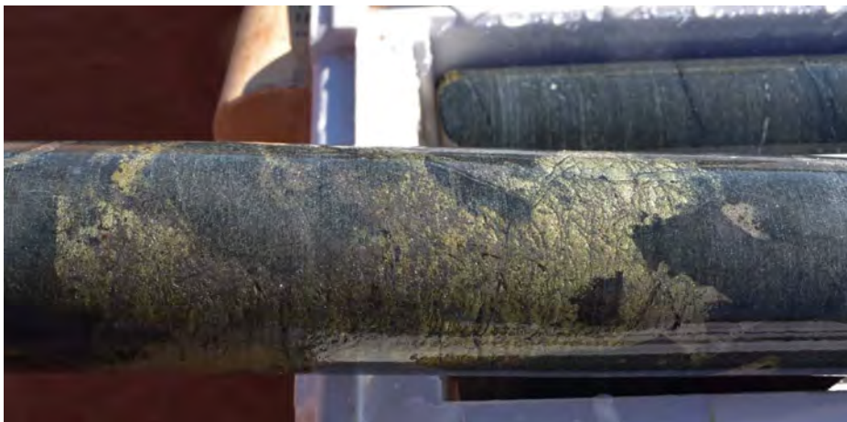
Figure 1 – photos of the drill core from MAD168 at approximately 230m downhole, showing breccia and stringer sulphides
