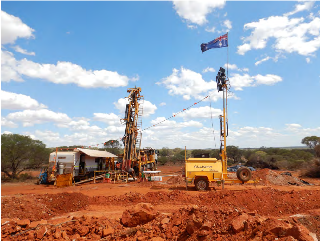
Above : diamond drill rig at Stricklands, Cathedrals Belt. Right : Drill core from MAD108.
