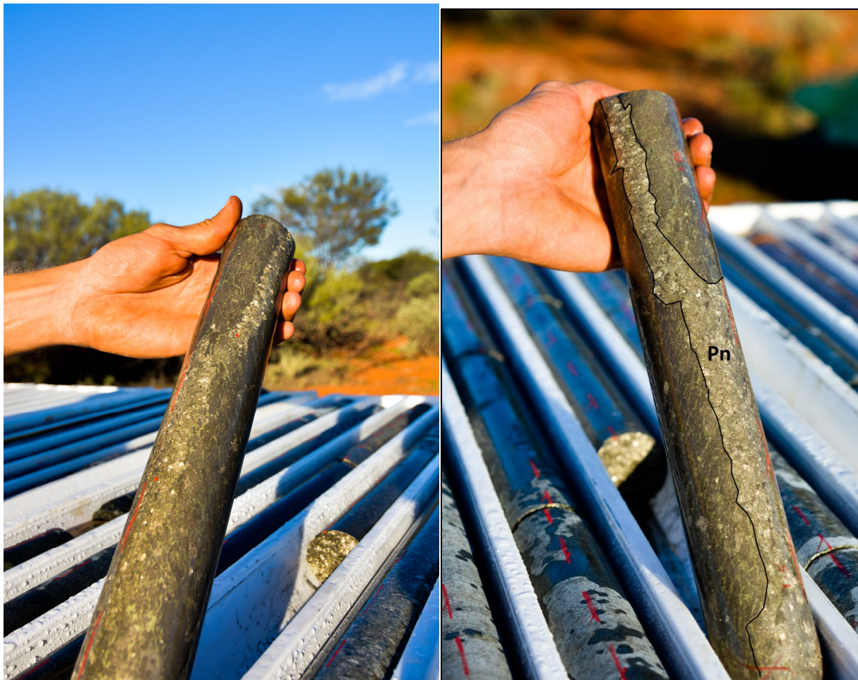
Figure 1 – photograph of drill core from MAD31 showing the pentlandite vein (outlined and labelled Pn in photo on left) that returned 28%Ni (based on XRF analysis) within the massive nickel-copper sulphide interval from 112.05-113.08.
