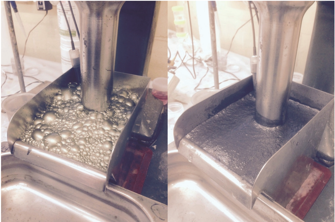
Figure 5 – photographs of a metallurgical flotation test on the Mt Alexander massive sulphide. On left: copper flotation test, with concentrates up to 32%Cu produced. On right: nickel flotation test, with concentrates up to 18%Ni produced.
