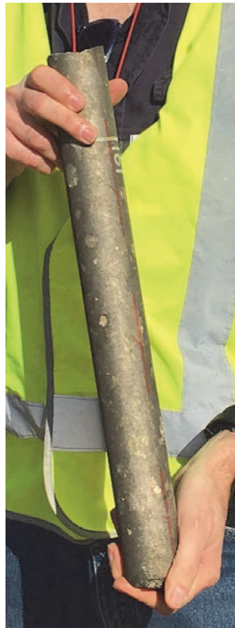
Figure 3 – drill core from MAD60 with large pentlandite crystals prominent in the core. The section of core displayed is from an interval that returned assays of 3m @ 6.40%Ni, 3.55%Cu, 0.21%Co and 5.25g/t total PGEs from 159.38m.
