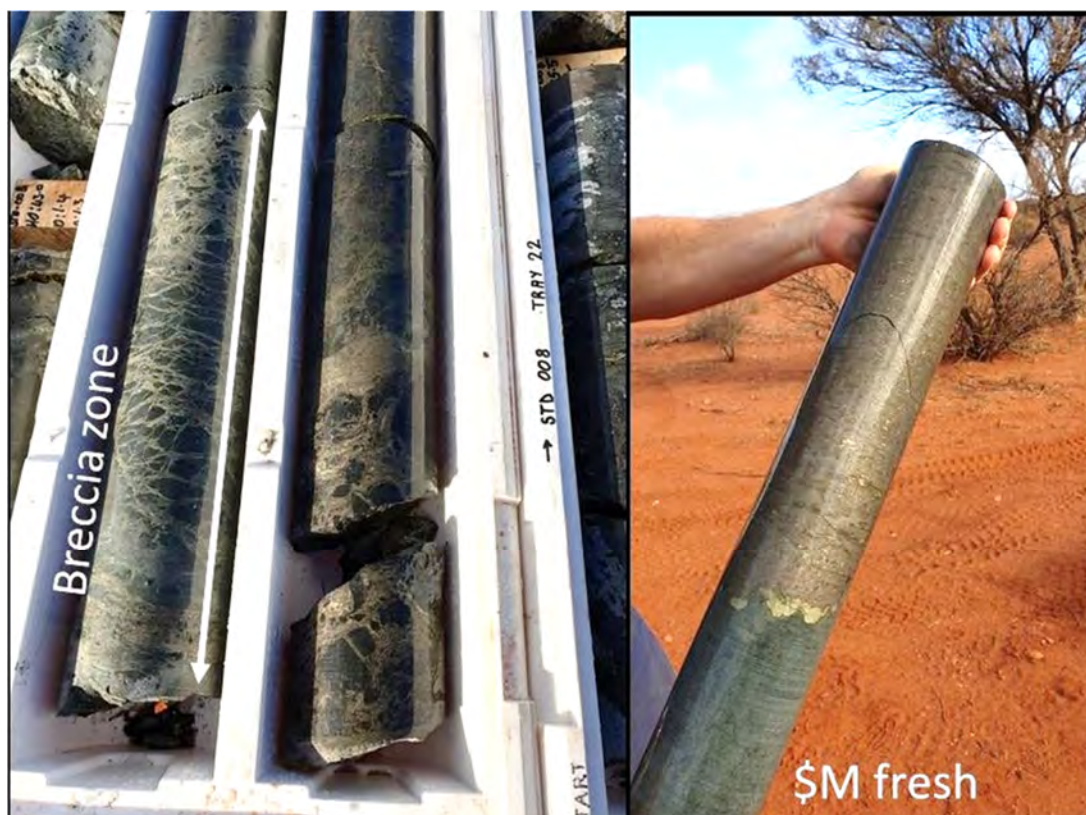
Figure 6 – photographs of drill core from STD008, one of the metallurgical holes completed at Stricklands. STD008 intersected 14.05m of nickel-copper sulphides from 36.7m downhole. The mineralised interval included massive sulphides (90-100% sulphides) between 36.7m to 46m (photo on right) and brecciated textured sulphides (50-75% sulphides) from 46m to 50.75m (photo on left).
