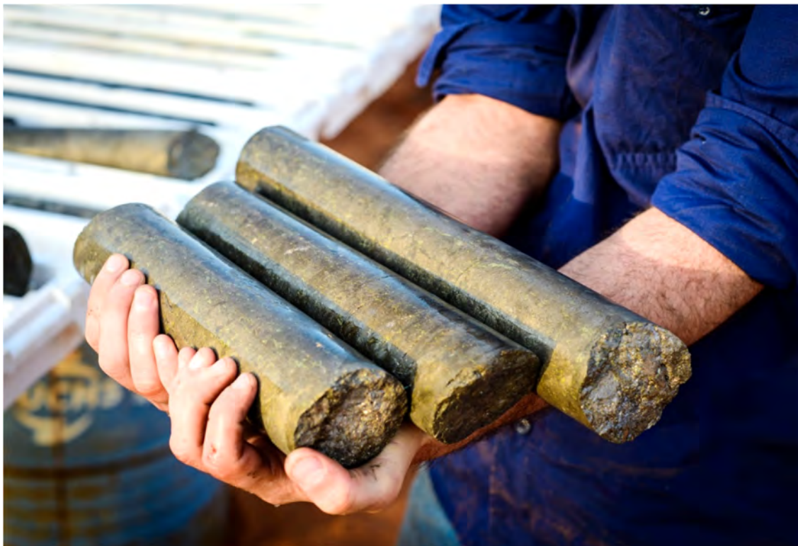
Figure 1 – drill core from MAD152 with massive sulphides intersected from 49.05m downhole.
