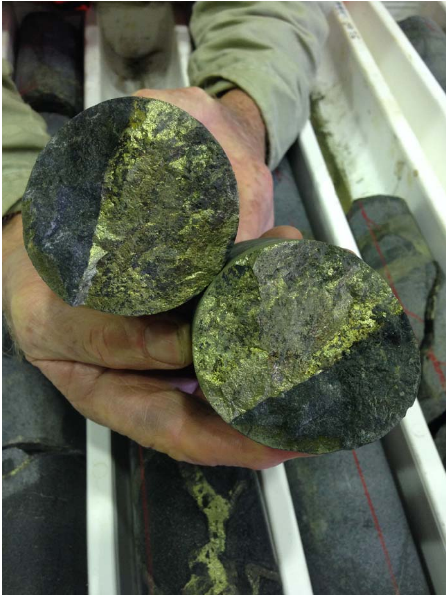
Figure 2 – drill core from MAD22 with massive chalcopyrite (yellow-green) in contact with ultramafic (dark grey). Assays for this interval (52.4m to 52.63m) returned 13.1%Cu and 43g/tAg.
