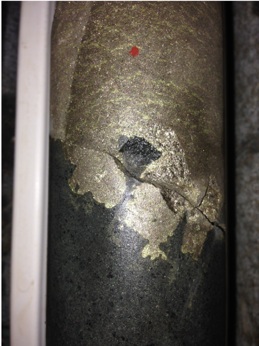
Figure 4 – primary igneous contact of massive nickel-copper sulphides against footwall mafics in MAD23 (57.7m). Lobate plumes of massive sulphide have projected into the footwall mafic and indicate in situ ultramafic-mafic contact.
