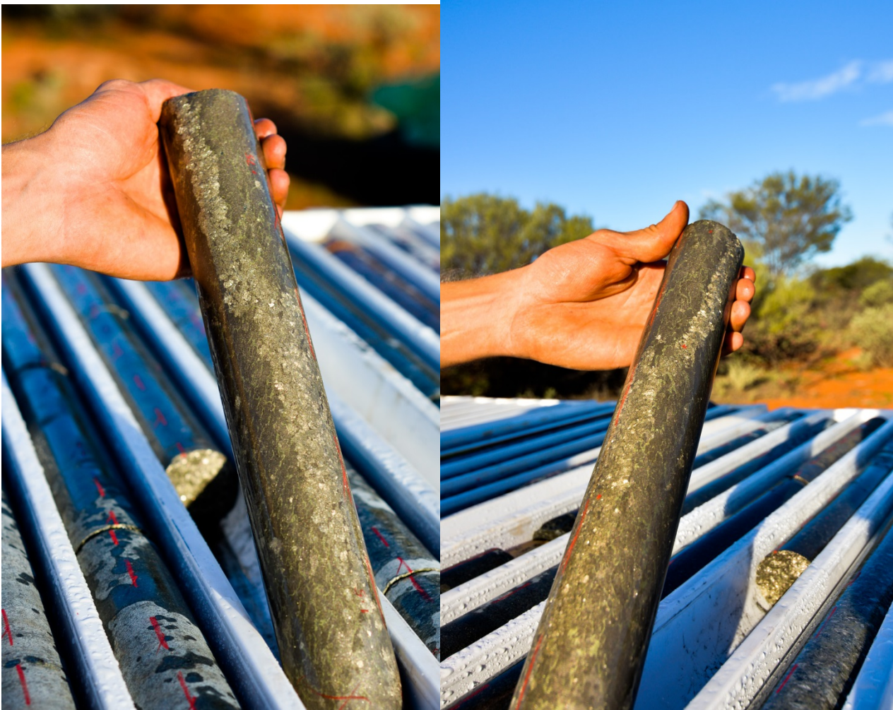
Figure 3 - drill core from MAD31 showing coarse grained pentlandite within the massive nickel-copper sulphide interval with assays of 1.57m @ 6.26%Ni, 2.71%Cu, 0.18%Co and 4.91g/t total PGEs from 111.67m.
