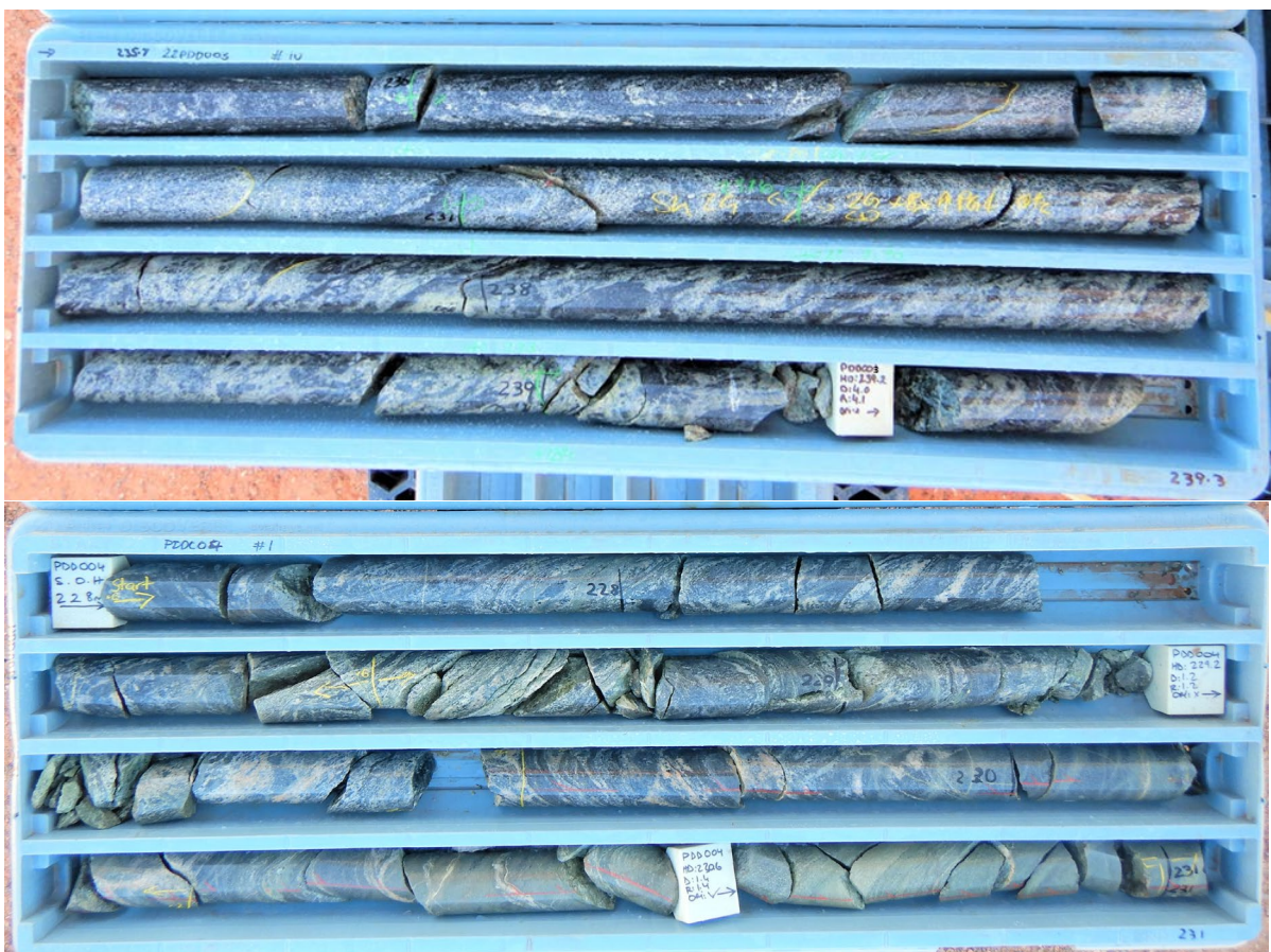
Figure 5: Photos of drill core from PDD003 (top) and PDD004 (bottom). Both showing brecciated zones with associated hydrothermal alteration.
