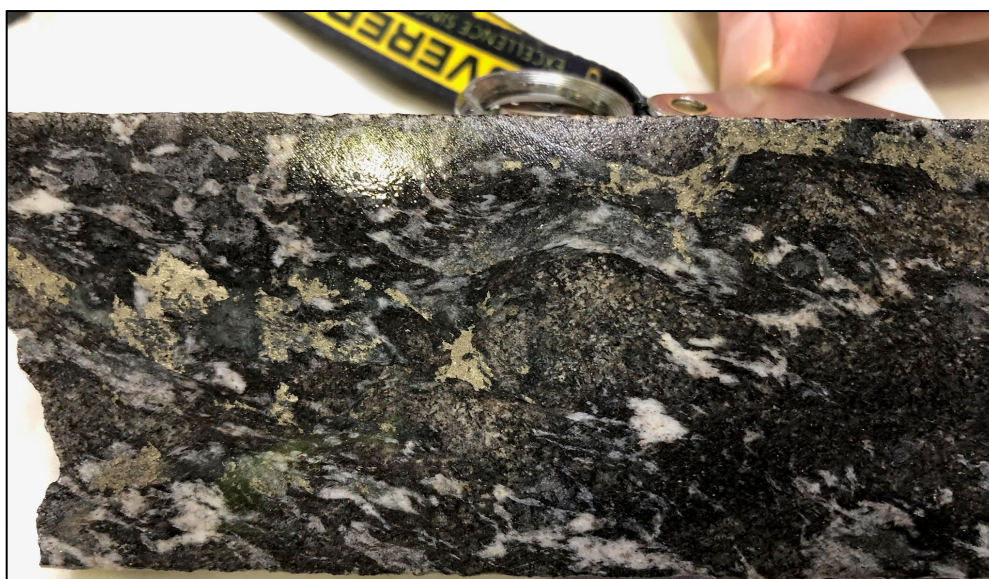
Figure 1: Core from PDD002 at 236m downhole showing disseminated and semi-massive sulphide (see Table 2) as void infill within an interpreted strongly altered breccia. Assays are pending.
