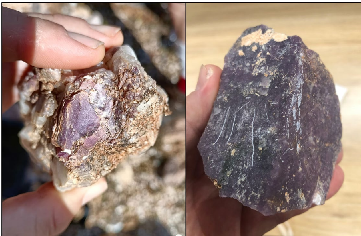
Figure 1 – photos of pegmatites from E29/962 (100% St George) with coarse grained purple crystals that may be indicative of spodumene and lepidolite, subject to confirmation by portable XRD spectrometer and laboratory analysis.
