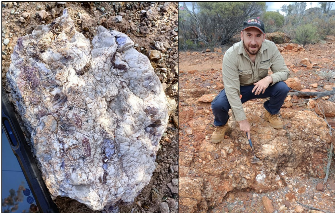
Figure 3 – photos of pegmatites from E29/962 (100% St George) including coarse grained purple crystals that may be indicative of spodumene and lepidolite, subject to confirmation by portable XRD spectrometer and laboratory analysis.
