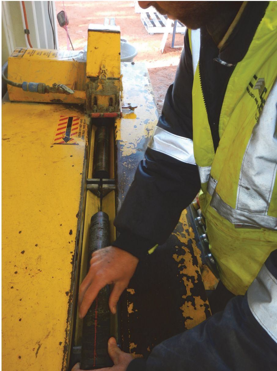
Figure 2 – cutting of drill core being completed at site in preparation for laboratory assays
