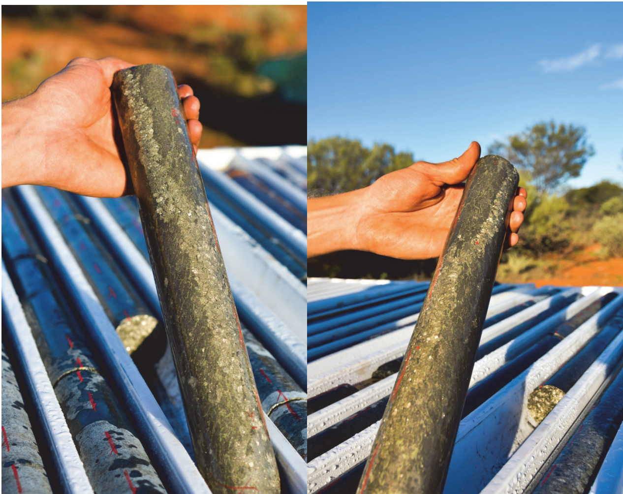
Figure 1 - drill core from MAD31 showing coarse grained pentlandite within massive nickel-copper-PGE sulphides with assays of 1.57m @ 6.26%Ni, 2.71%Cu, 0.18%Co and 4.91g/t total PGEs from 111.67m.
