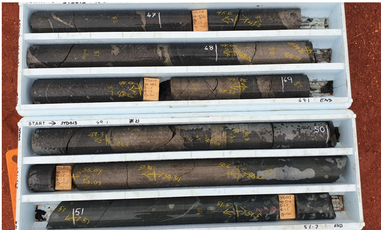
Figure 5 – core tray for STD013 showing mineralised interval with massive sulphides between 47.2m and 50.6m downhole.
