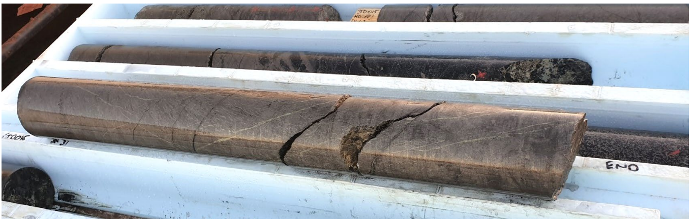
Figure 3 – drill core tray for STD015 showing massive sulphides intersected from 67.3m downhole.
