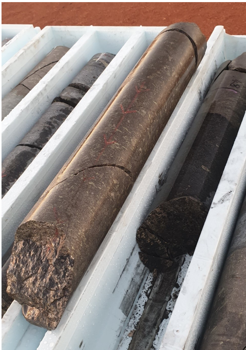
Figure 4 – drill core from STD014 showing massive sulphides intersected from 48.2m to 48.9m downhole. STD014 intersected a 14.1m thick interval of sulphide mineralisation from 36.5m downhole.
