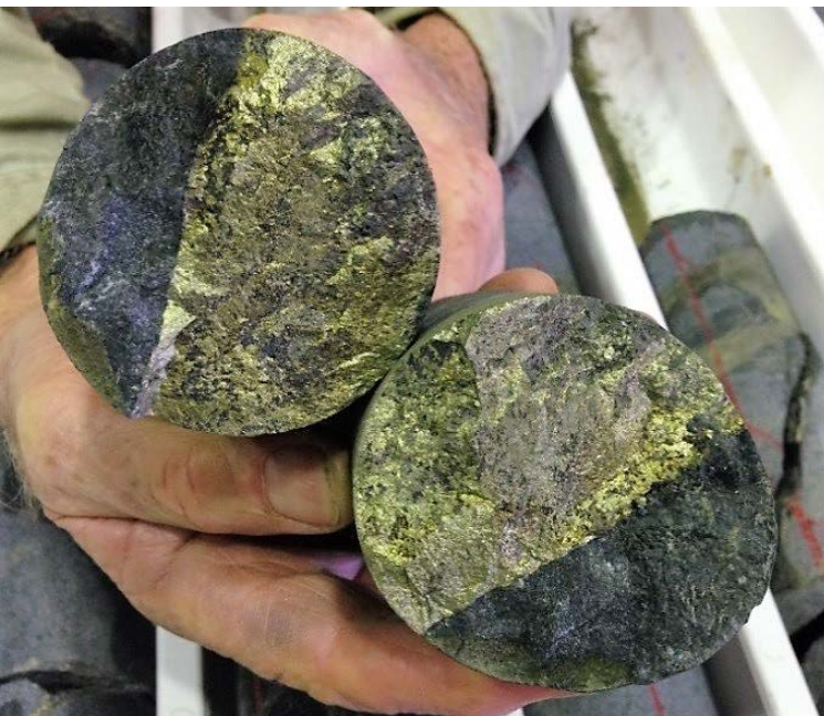
Left: drill core from MAD22 with massive chalcopyrite (yellow-green) in contact with ultramafic (dark grey). Assays for this interval (52.4-52.6m) are 13.1%Cu and 43g/tAg. Above: Cathedrals Belt (against high resolution TMI) showing the multiple intersections of massive nickel-copper-cobalt-PGE sulphides (“$M”) over a strike length of 3.5km and new regional targets.
