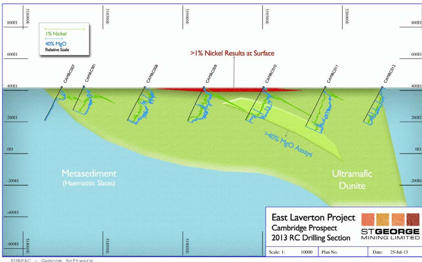
Figure 2- Drill section across the Cambridge ultramafic body shows the highest Ni values (green lines) and MgO values (blue lines) in the central zone. The MgO content of the ultramafic increases with depth and dips to the east. The deepest contact with this easterly dipping high-MgO zone is made in CAMRC-011, which intersects 42 m @ 0.26%Ni and 40.1 % MgO at the base of the hole, and appears to have encountered the top of an olivine adcumulate zone.
