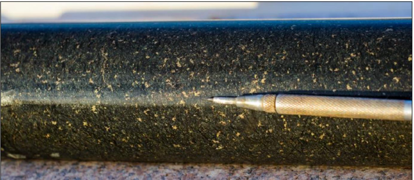
**Figure 1:** Drill-core with heavily disseminated sulphides from the interval at 46.3m to 48.7m downhole in MAD152 at the Radar Prospect
